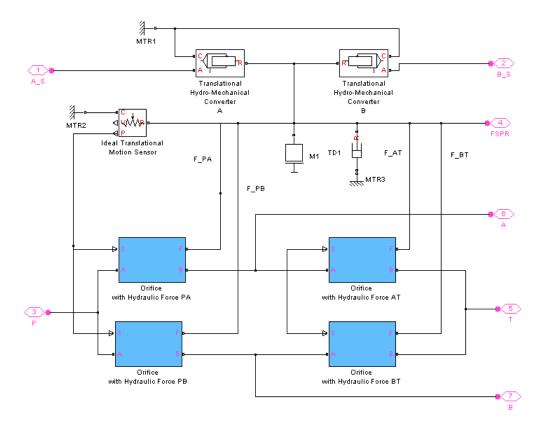
The spool (mass M1, viscous friction TD1) is shifted by the servo-actuator simulated by two Translational Hydro-Mechanical Converter blocks. Connections  $A\_S$  and  $B\_S$  are hydraulic ports for applying pilot control pressure.
