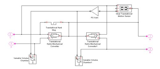
Connections R and C are mechanical translational conserving ports corresponding to the cylinder rod and cylinder clamping structure, respectively. Connections A and B are hydraulic conserving ports. Port A is connected to chamber A and port B is connected to chamber B.
