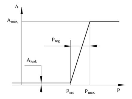
The valve remains closed while pressure at the valve inlet is lower than the valve preset pressure. When the preset pressure is reached, the value control member (spool, ball, poppet, etc.) is forced off its seat, thus creating a passage between the inlet and outlet. Some fluid is diverted to a tank through this orifice, thus reducing the pressure at the inlet. If
