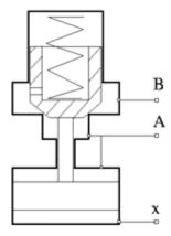
Unlike a conventional check valve, the pilot-operated check valve can be opened by inlet pressure  $p_A$ , pilot pressure  $p_X$ , or both. The force acting on the poppet is determined as
