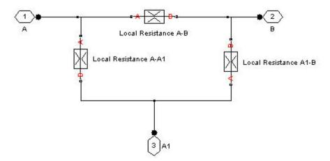
To specify pressure loss for all possible flow directions, you have to provide six pressure loss coefficients.
