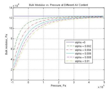
Cavitation is an inherently thermodynamic process, requiring consideration of multiple-phase fluids, heat transfers, etc., and as such cannot be accurately simulated in SimHydraulics. But the simplified
