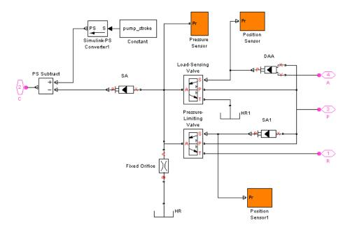
There are three hydraulic valve actuators in the model:
