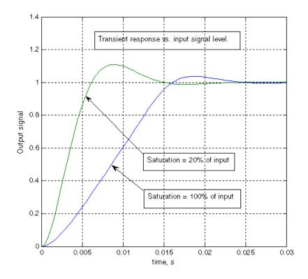
You can adjust the block parameters, such as saturation, gain, and time constant, to make the transient responses close enough to those provided in the data sheet. The most effective way to adjust the parameters is to use Simulink Response Optimization Toolbox.
