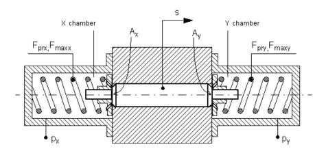
As pressure applied to the piston develops enough force to overcome the spring preload, the piston moves to the opposite position until it reaches its maximum stroke. Pressure applied at port X shifts the valve in the x-direction, overcoming the spring located in the Y chamber. Pressure
