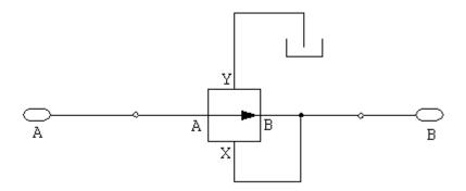
The block positive direction is from port A to port B. This means that the flow rate is positive if it flows from A to B, and the pressure differential is determined as  $p = p_A - p_B$ .
