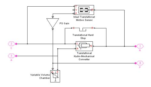
Connections R and C are mechanical translational conserving ports corresponding to the cylinder rod and cylinder clamping structure, respectively. Connection A is a hydraulic conserving port associated
