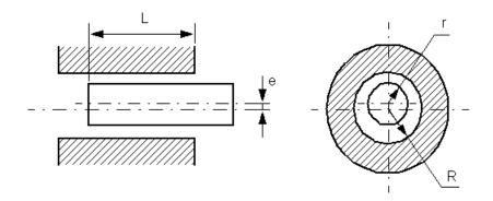
The flow rate is computed using the Hagen-Poiseuille equation (see [1]):
