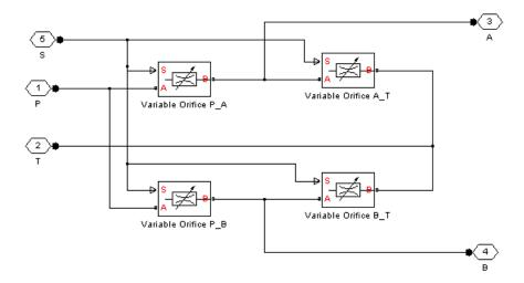
The Variable Orifice blocks are installed as follows: orifice\_PA is in the P-A path, orifice\_PB is in the P-B path, orifice\_AT is in the A-T path, and orifice\_BT is in the B-T path. All blocks are controlled by the same position signal, provided through the physical signal port S, but the **Orifice orientation** parameter in the block instances is set in such a way that positive signal at port S opens orifice PA and
