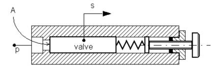
The actuator consists of a piston and a spring. The spring, which can be preloaded, tends to keep the piston at the initial position. As pressure applied to the piston develops enough force to overcome the spring preload, the piston moves to the opposite position until it reaches its maximum stroke.
