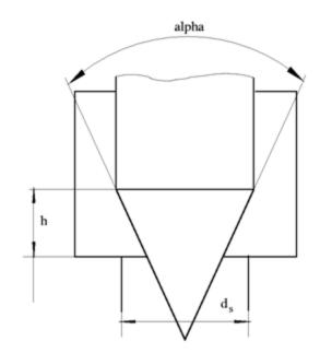
The flow rate through the valve is proportional to the valve opening and to the pressure differential across the valve. The model accounts for the laminar and turbulent flow regimes by monitoring the Reynolds number (Re) and comparing its value with the critical Reynolds number (Re $_{cr}$ ). The flow rate is determined according to the following equations:
