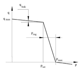
The pump tries to maintain preset pressure at its outlet by adjusting its delivery flow in accordance with the system requirements. If pressure differential across the pump is less than the setting pressure, the pump outputs its maximum delivery corrected for internal leakage. After
