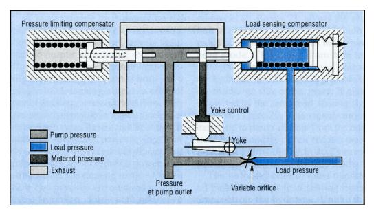
The Hydraulic Actuator with Load-Sensing Variable-Displacement Pump demo (sh\_hydraulic\_actuator\_load\_sensing\_pump) implements this type of control. The next illustration shows the schematic of the Load-Sensing and Pressure-Limiting Control block in the demo.
