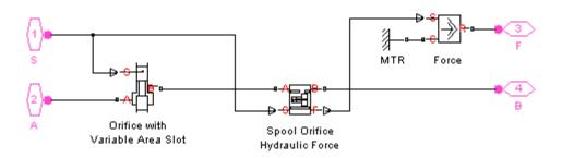
It consists of an Orifice with Variable Area Slot block, which simulates hydraulic properties of the orifice, connected in series with a Spool Orifice Hydraulic Force block. The force value computed in the block is exported through its port F and passed to the Force block.
