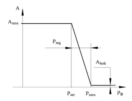
The pressure-reducing valve is a normally open valve and it remains fully open while outlet pressure is lower than the valve preset pressure. When the preset pressure is reached, the value control member (spool, ball, poppet, etc.) is forced off its stop and starts closing the orifice, thus
