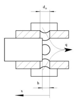
The model accounts for the laminar and turbulent flow regimes by monitoring the Reynolds number (Re) and comparing its value with the critical Reynolds number  $(Re_{cr})$ . The flow rate is determined according to the following equations:
