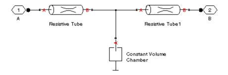
The Resistive Tube blocks account for friction losses, while the Constant Volume Chamber block accounts for fluid compressibility. By using the block parameters, you can set the model to simulate pipeline with rigid or compliant walls, including simulation of hydraulic hoses with elastic and viscoelastic properties.
